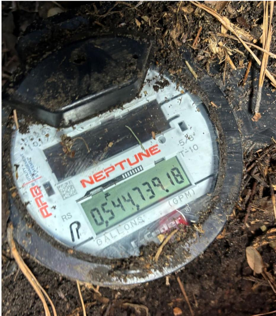
When the screen toggles, the rate of flow is visible and is shown in gallons per minute for four seconds. Then it toggles back to the read screen.
